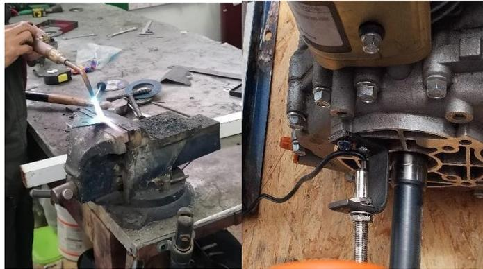
(b) Acople sensor RPM
