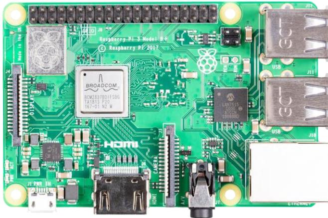
Raspberry Pi 3 Model B+ has a 64-bit quad-core processor running at 1.4GHz, dual-band 2.4GHz and 5GHz wireless LAN, Bluetooth 4.2/BLE, Gigabit Ethernet over USB 2.0, and PoE capability via a separate PoE HAT. The dual-band wireless LAN comes with modular compliance certification.
